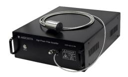
The HPSL High Power Single Mode Laser is a user-friendly benchtop unit that delivers up to 20W single mode and 10W polarization Maintain stable laser output. The output is in CW mode or in a variable-modulated mode with a frequency of up to 10kHz. The output is a collimator with a built-in isolator. It has a front power control knob and USB computer interface. An emission switch adds safety.
